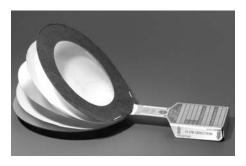
The ENVIRO-SEAL Type II Rupture Disc is designed to burst in either the positive or vacuum direction, at the same burst pressure. Seal material is located on both the vent and the process sides of a single top section, providing a completely lined rupture disc. This feature provides a durable corrosion barrier from both process media and atmospheric corrosives while maintaining dual direction protection.
