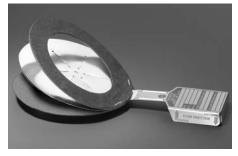
The ENVIRO-SEAL Type III Rupture Disc is also designed to burst in either the positive or vacuum direction at the same burst pressure. However, the ENVIRO-SEAL Type III Rupture Disc consists of two metallic top sections, one located on the process side and one on the vent side of the rupture disc. A single seal is located between the two top sections.
